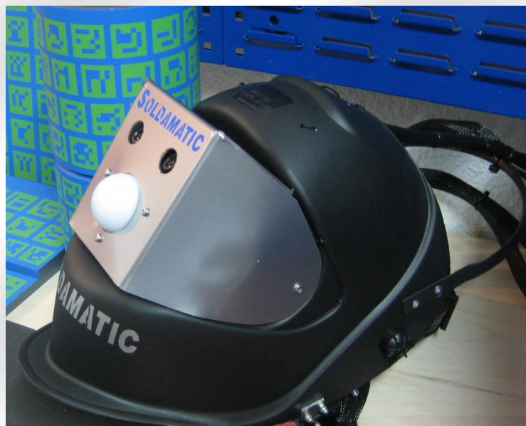
Welding mask with micro-cameras and 3D Video Glasses inside
